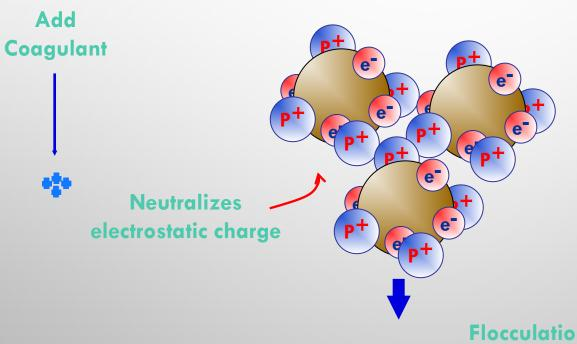
**Once suspended** particles are flocculated into larger particles, they can usually be removed from the liquid by settling, filtering, or centrifuging.
